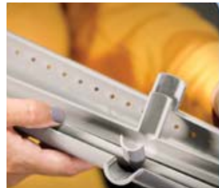
Completely disassemble the distribution tube.
