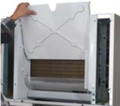
Remove the evaporator splash plate.
